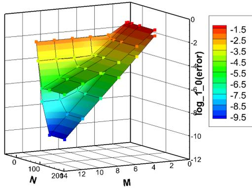
Figure 3: Approximate method:  $k.h = 0.916$ ,  $k.a = 0.1$ . Influence of  $\frac{\beta}{h_0}$  on error on  $W$  ( $\log(\epsilon_w)$ ) as function of  $N$  and  $M$ . Low-surface:  $\frac{\beta}{h_0} = 0\%$ , high:  $\frac{\beta}{h_0} = 25\%$
