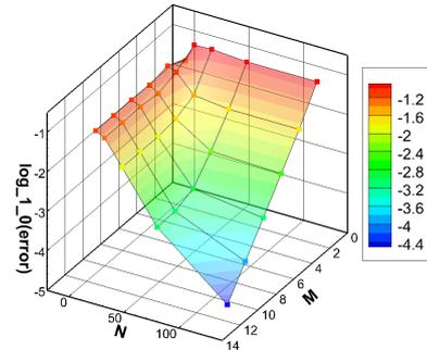
Figure 2: Exact method:  $k.h = 0.916$ ,  $k.a = 0.2$ , all  $\frac{\beta}{h_0}$ . Error on  $W$  ( $\log(\epsilon_w)$ ) as function of  $N$  and  $M$ .
