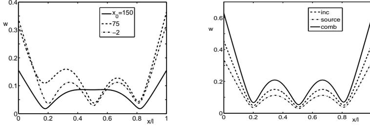
In the figure on the left hand side the deflection, of the platform, induced by a point source at the location indicated is shown. The length of the platform is 300 m.,  $\mathcal{D} = 10^7 \text{ m}^4$  and  $\frac{\omega^2}{g} = 2\pi/60$ , hence the *deep water* wavelength is 60 m. The figure on the right hand side
