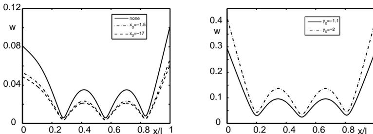
The deflection is shown in the figure on the left for  $\frac{\omega^2}{g} = 2\pi/30$  and two values of  $x_0$  and fixed  $y_0 = -1.5$ , while the one on the right shows results for  $\frac{\omega^2}{g} = 2\pi/60$  and different values of  $y_0$  and fixed  $x_0 = -1.5$ .
