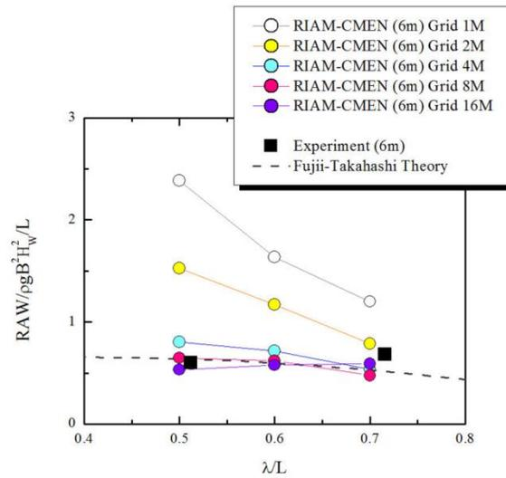
Fig.2 Grid convergence test on added resistance
