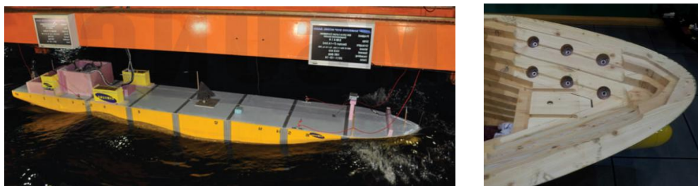
Fig.3 Model experiment for a 18,000TUE containership and installed pressure sensors at SSMB
