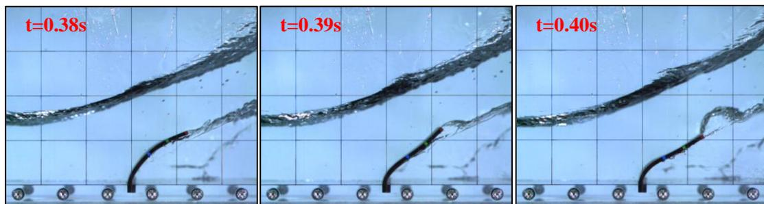
Fig.1 Structural second-order vibration modes
