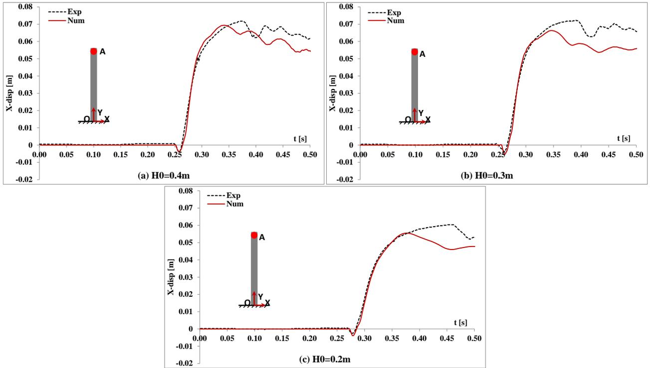
Fig.4 Time history of X-displacement at point A
