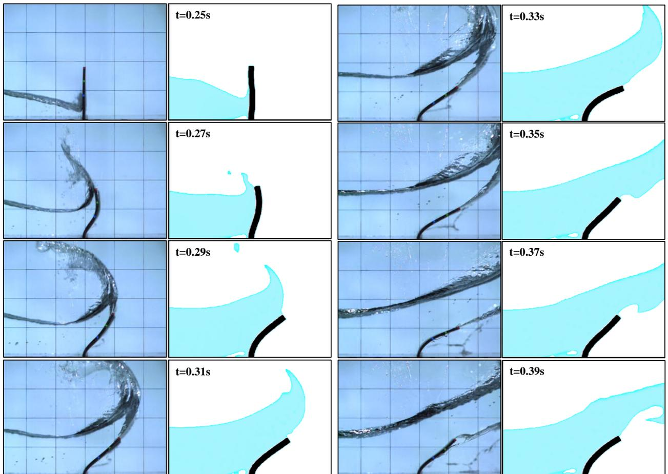
Fig.5 Free surface profile and structural deformation ( $H_0=0.4\text{m}$ )
